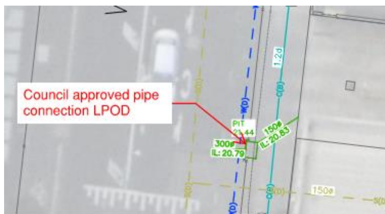
Figure 7 Council pit LPOD for piped connection
