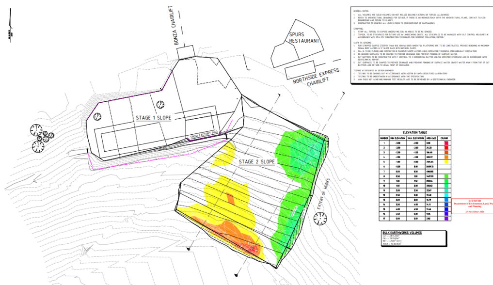
Figure 9: Stage 2 slope regrading (Source: Application)
