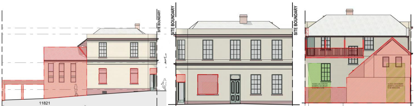
Figure 14: Extent of external demolition and works – western (Star Street), southern (Myers Street) and northern (rear) views
