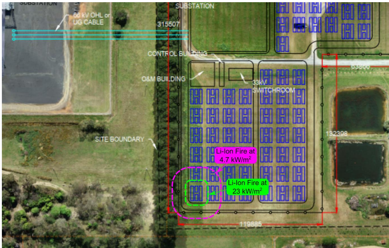
Figure 6-1: Li-Ion Battery Module Fire Radiant Heat Contours
