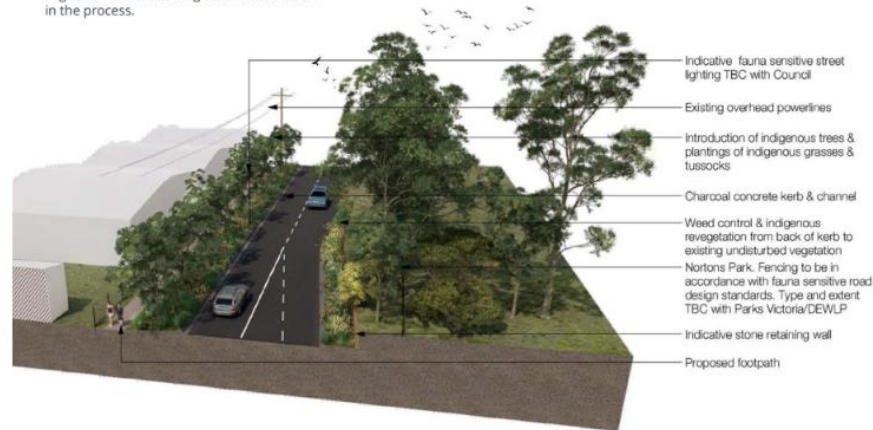
Figure 17 - Indicative Nortons Lane Cross-Section looking south towards Development Plan area. Subject to minor changes.
