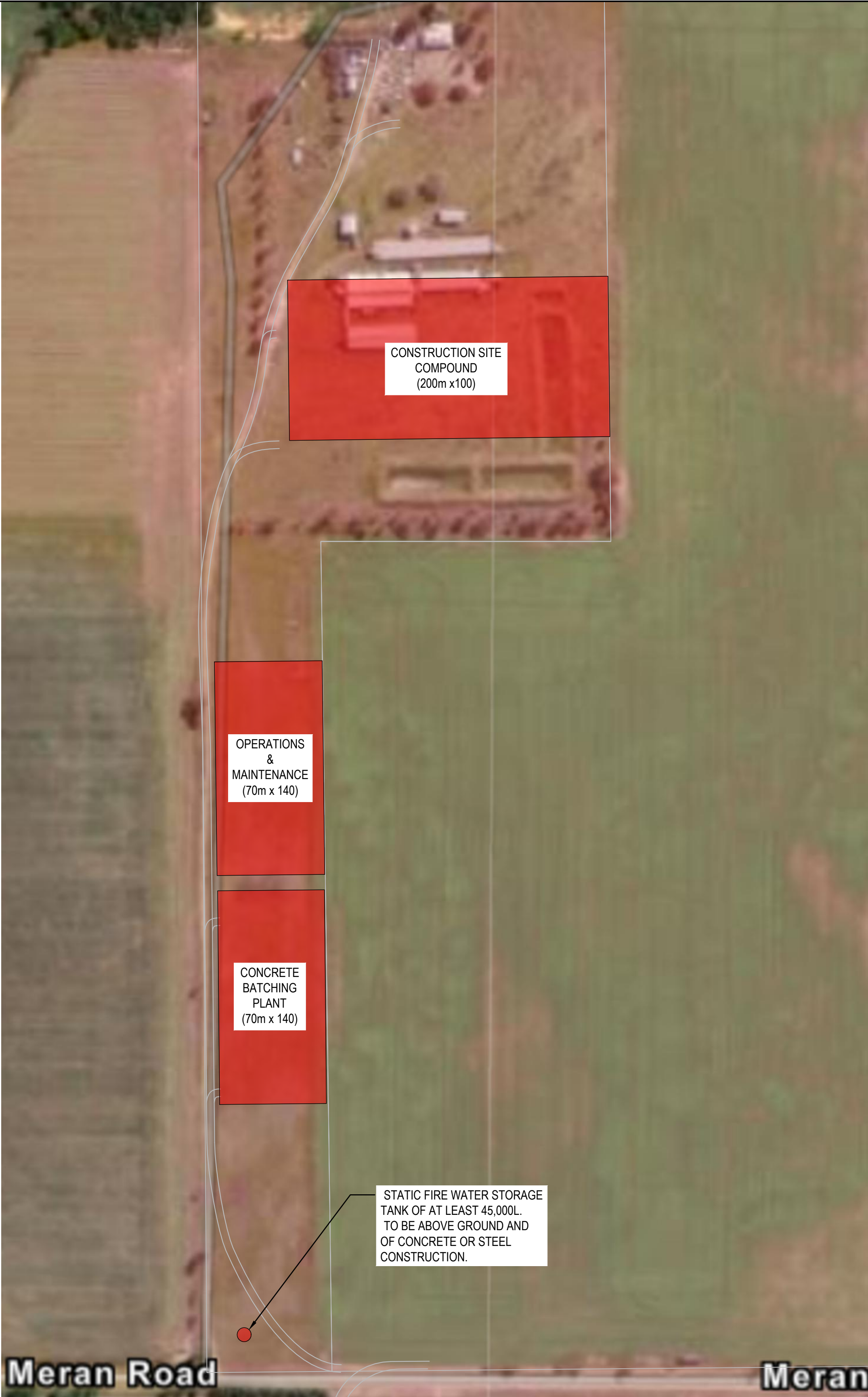
PROPOSED SITE LOCATION - PLAN SCALE: 1:2000
