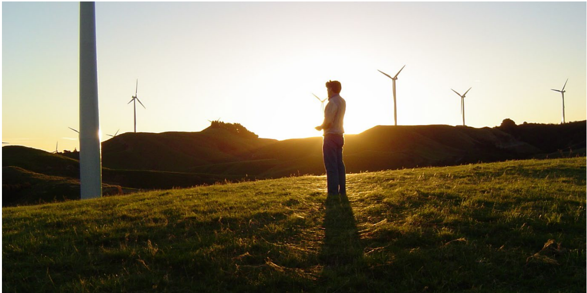
Figure 4-2 Diffuse sunlight at low sun elevation angle, resulting in insignificant shadow flicker effects
