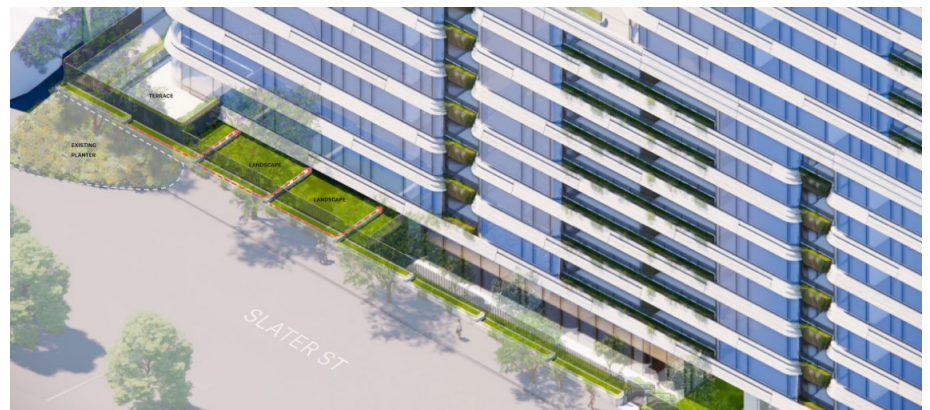
Figure 32: Axo diagram to illustrate the setbacks and Level 1 terrace adjacent to the existing street planter along Slater Street
