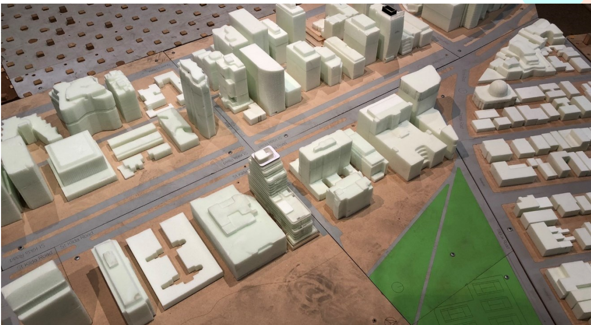
Figure 4 – View from the southeast of the 1/400 scale Proposed Configuration model of the 437 St Kilda Road Development in the wind tunnel.
