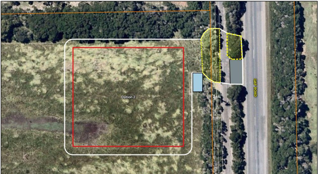
Figure 8: Option 2 showing the indicative construction footprint as white polygon. Red polygon indicate approximate location of the battery storage facility, yellow dotted areas indicate native vegetation removal, grey area indicate culvert location, blue polygon show existing water pumping station, orange line indicate cadastral boundaries.
