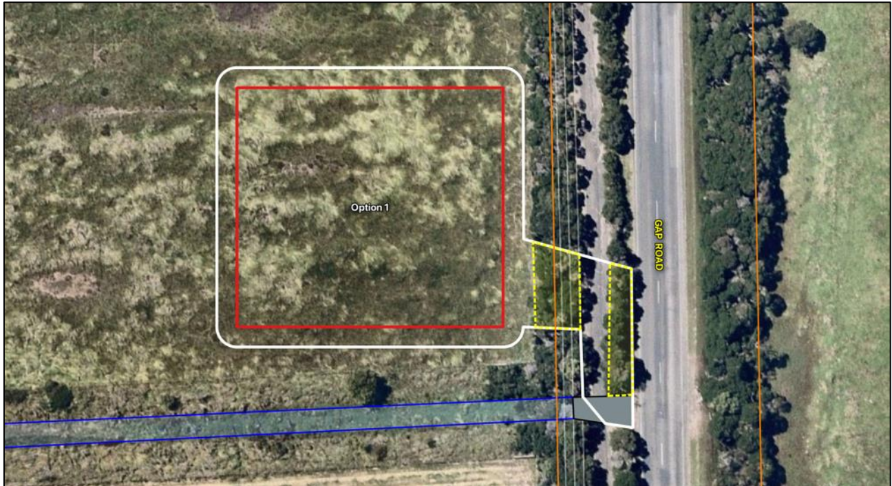
Figure 3: Option 1 showing the indicative construction footprint as white polygon. Red polygon indicate approximate location of the battery storage facility, yellow dotted areas indicate native vegetation removal, grey area indicate culvert location, blue polygon show indicative location of the watercourse, orange line indicate cadastral boundaries.
