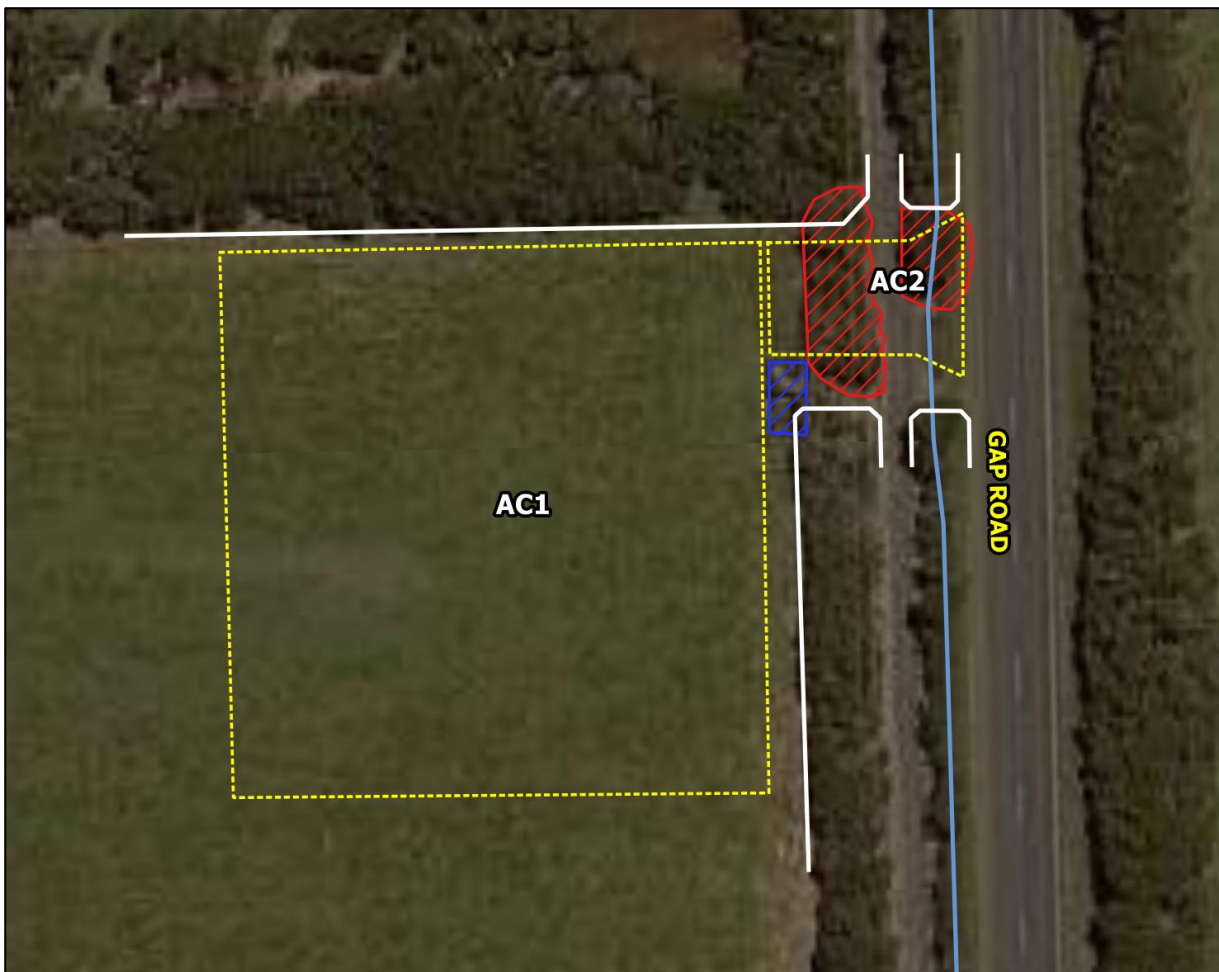
Figure 2: Site plan. Dashed yellow lines indicate construction footprint, white lines indicate location of vegetation protection fencing, red hashed areas indicate areas of native vegetation to be removed, blue hashed area indicates existing pumping station, light blue line indicates roadside drain.
