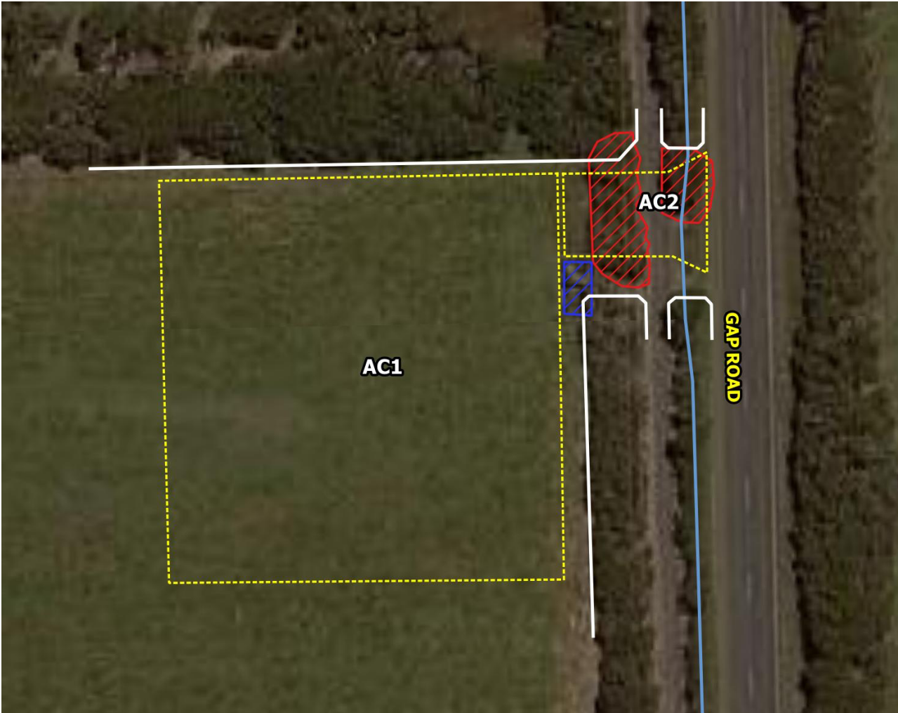
Figure 4: Site plan. Dashed yellow lines indicate construction footprint, white lines indicate location of vegetation protection fencing, red hashed areas indicate areas of native vegetation to be removed, blue hashed area indicates existing pumping station, light blue line indicates roadside drain.
