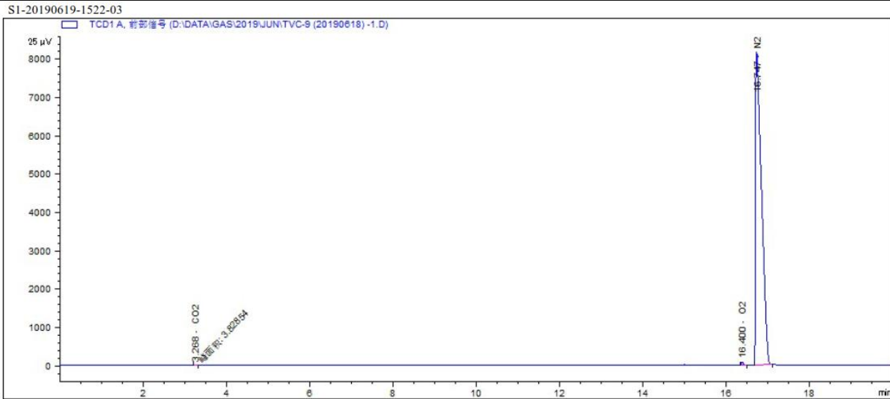
GC-MS spectrogram analysis for gas released after test: cell sample ID: 0818CAS01064
