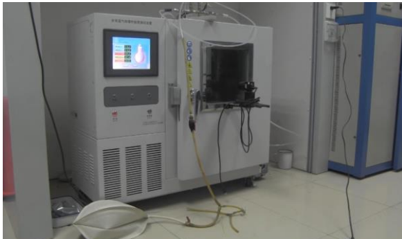
Gas Mixture During LFL Testing.
