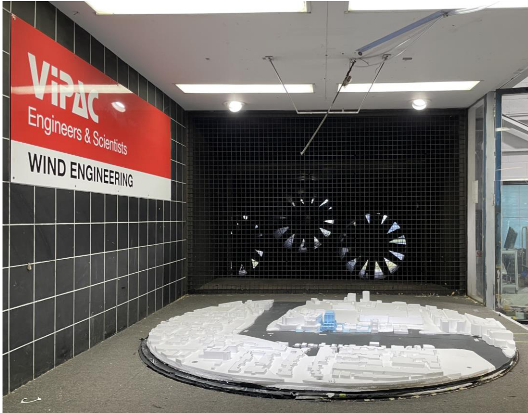
Figure 5: Overall view from northwest of the 1:400 scale model of the proposed development in the wind tunnel.
