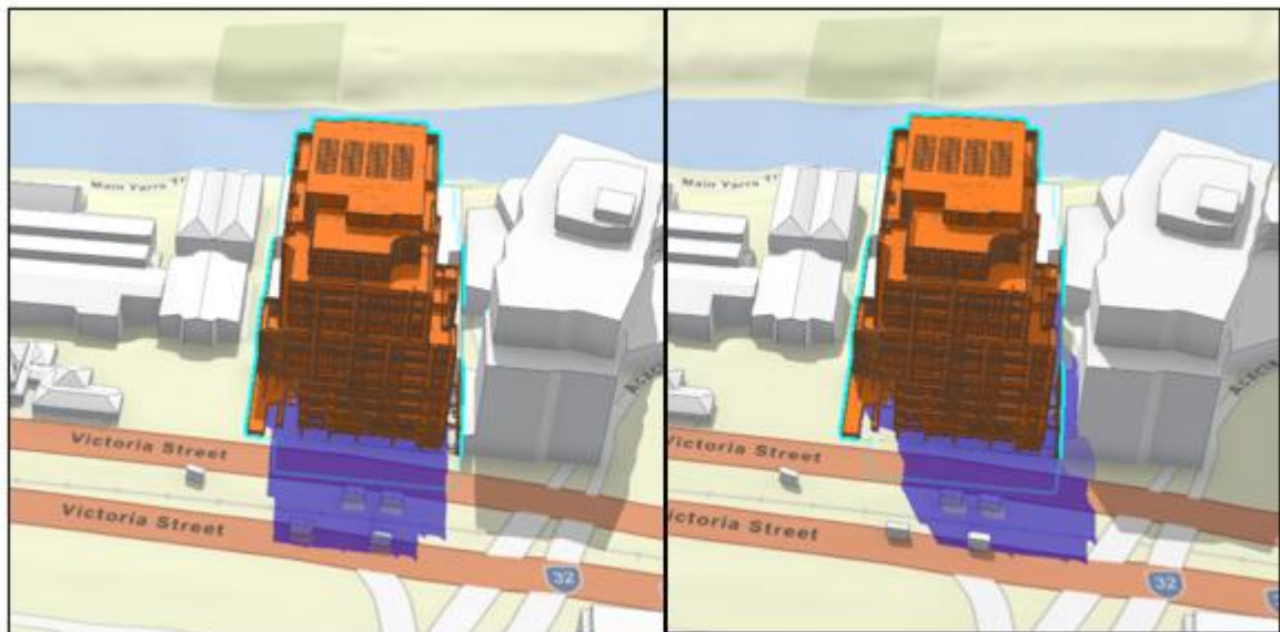
Figure 26: Shadow study 22 September 12pm (left image) and 1pm (right image) (Source: DTP)
