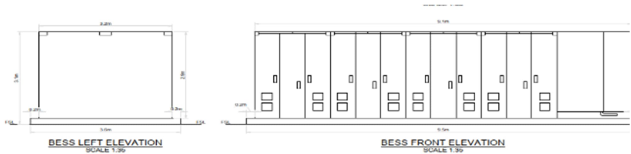
Figure 9 – Typical BESS Elevations
