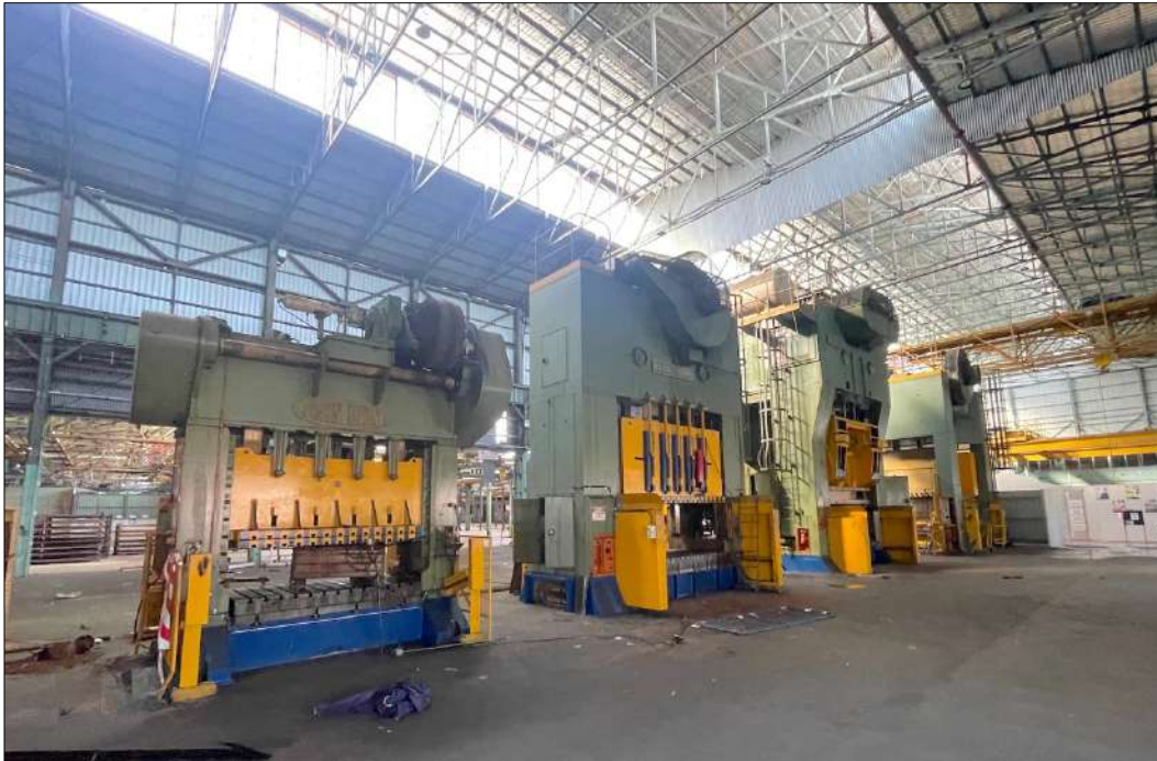
Figure 44 Mechanical presses inside the crane bay.
