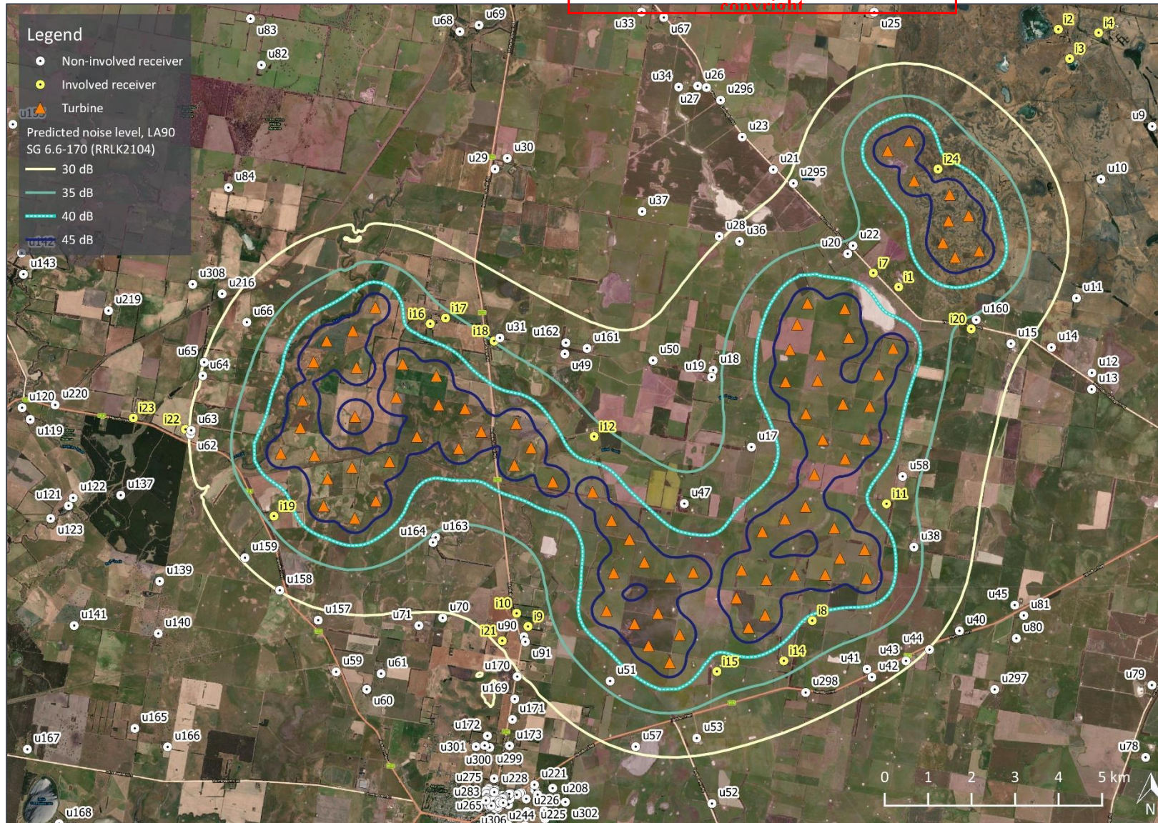
Figure 1: Highest predicted noise level contours, dB LA90 – SG 6.6-170
