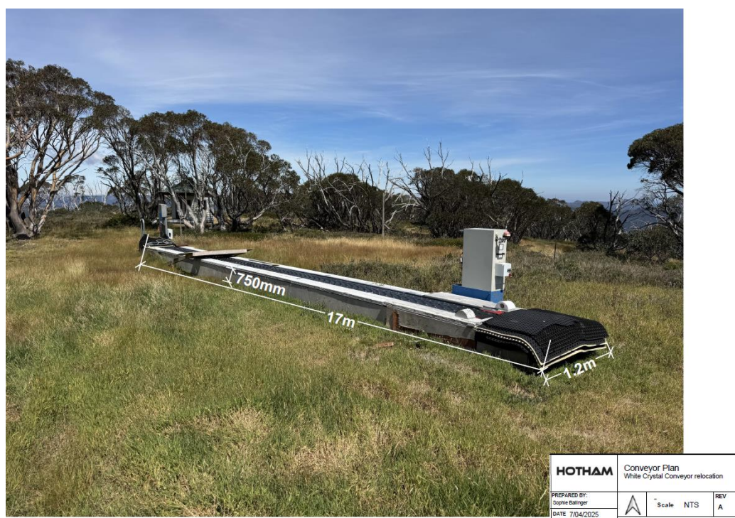
Figure 2: Existing ski conveyor in its existing Big D area (before it is relocated) (Source: Application)
