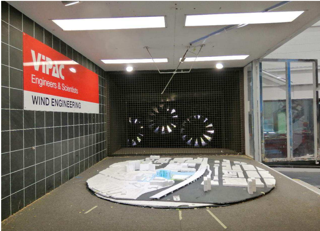
Figure 5: Overall view from north of the 1:400 scale model of the proposed development in the wind tunnel (Configuration 1)
