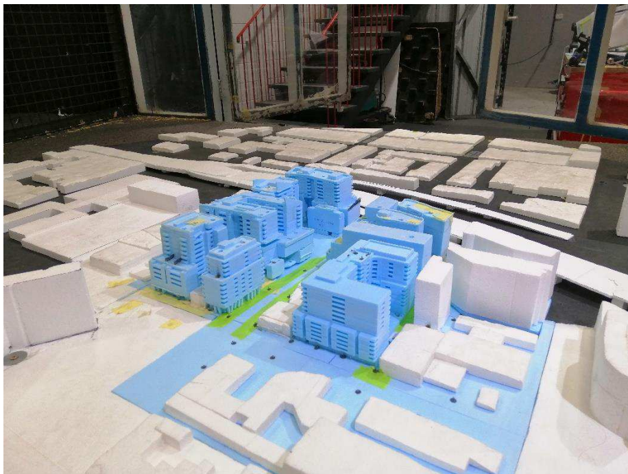
Figure 6: Close up view from the west of the 1:400 scaled model in the wind tunnel (Configuration 2).
