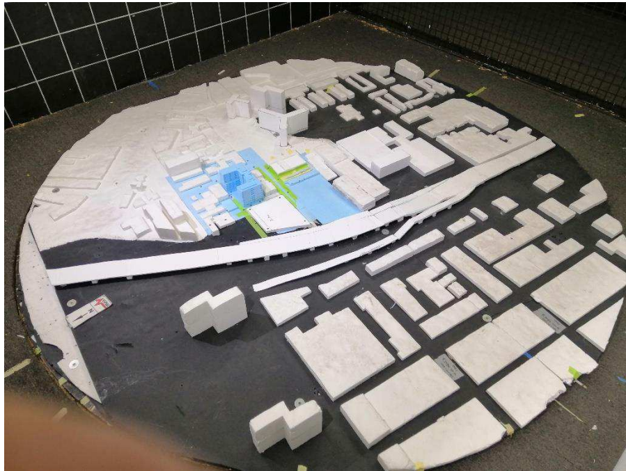
Figure 15: Overall view of the proposed development model in the wind tunnel (Configuration 1).
