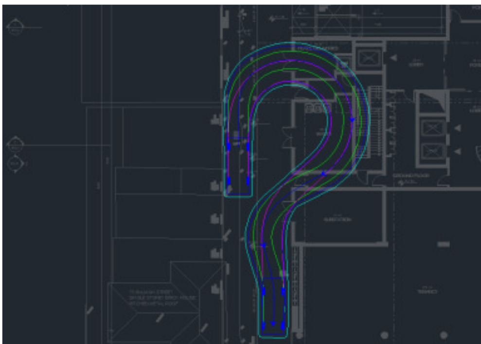
Figure 16: Required turning circle for porte-cochere
