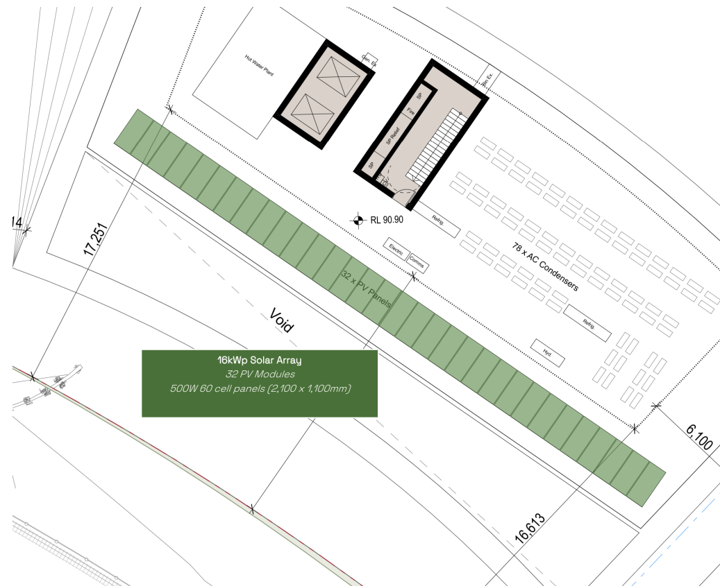
Figure 19 Track Central Solar Array
