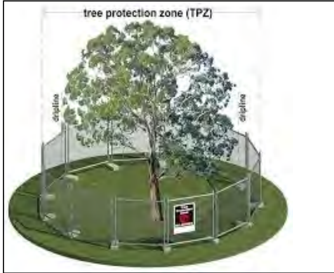
Figure 1. Steel mesh fencing is to be 1.8m temporary fence with weighted feet. Each panel is to be fastened together to deter entry and movement. Signage must be placed on the fencing and be clearly visible, reading "Tree Protection Zone". Fencing may be replaced with suitable trunk and ground protection system under guidance from the Project Arborist.
