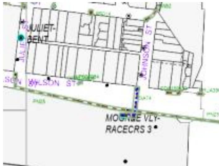
Figure 1.3: Incoming HV Cabling to Moonee VLY-Race CRS 3 Substation
