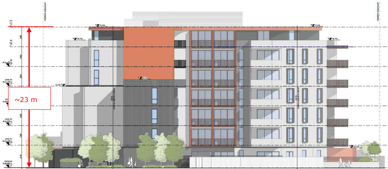
Figure 2: East elevation of the proposed development.
