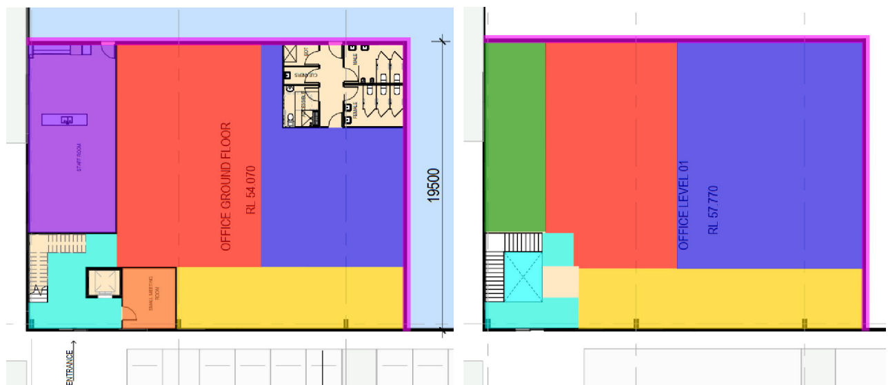
Figure 13: HVAC zones & thermal envelope for 16 McLaren Drive Ground Floor (Left) and First Floor (Right)
