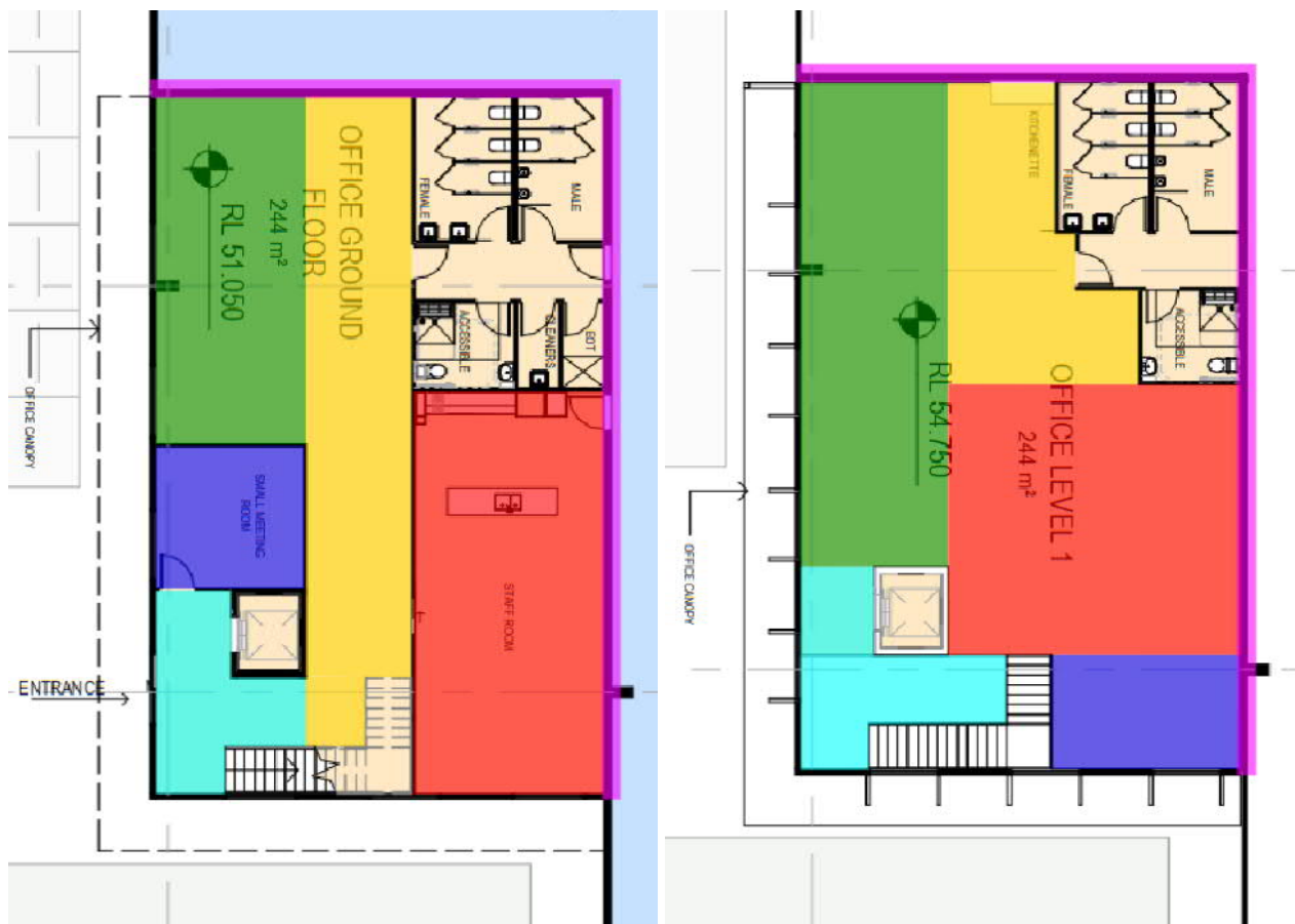
Figure 24: HVAC zones & thermal envelope for 2 McLaren Drive Ground Floor (Left) and First Floor (Right)
