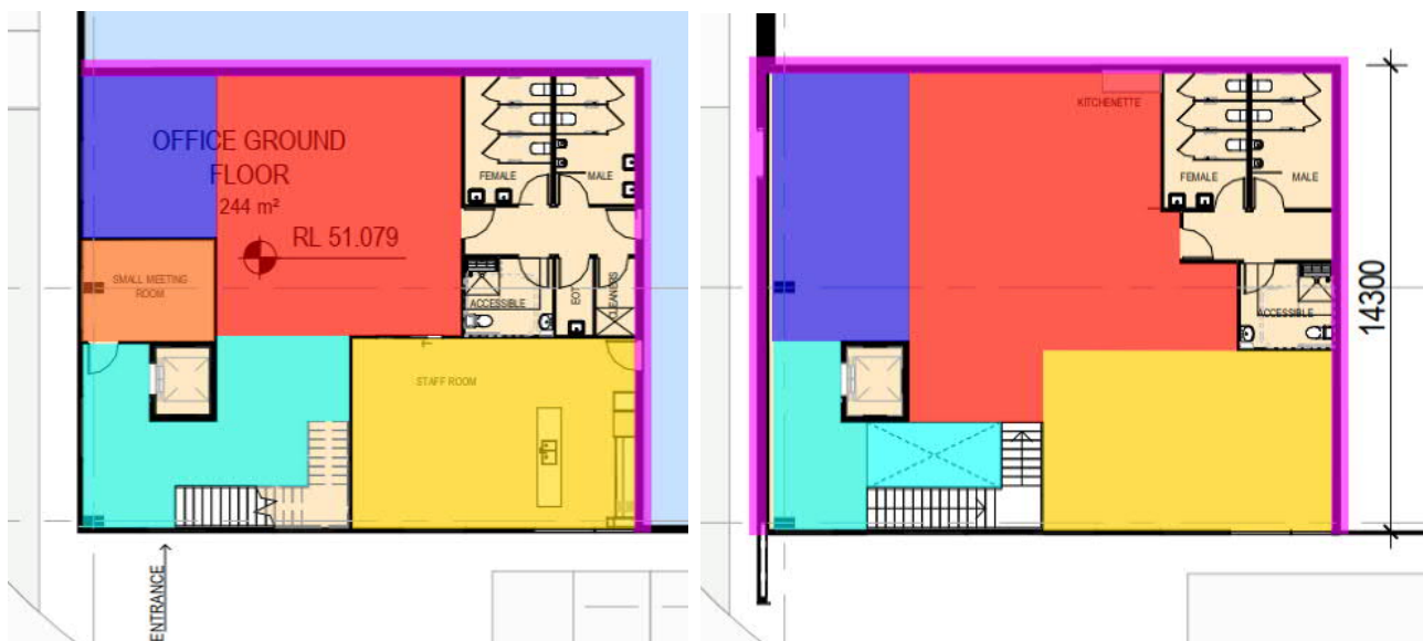
Figure 12: HVAC zones & thermal envelope for 12 McLaren Drive Ground Floor (Left) and First Floor (Right)
