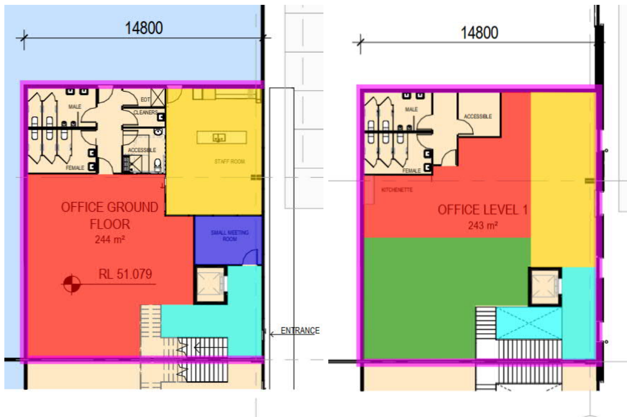
Figure 14: HVAC zones & thermal envelope for 3 Senator Drive Ground Floor (Left) and First Floor (Right)
