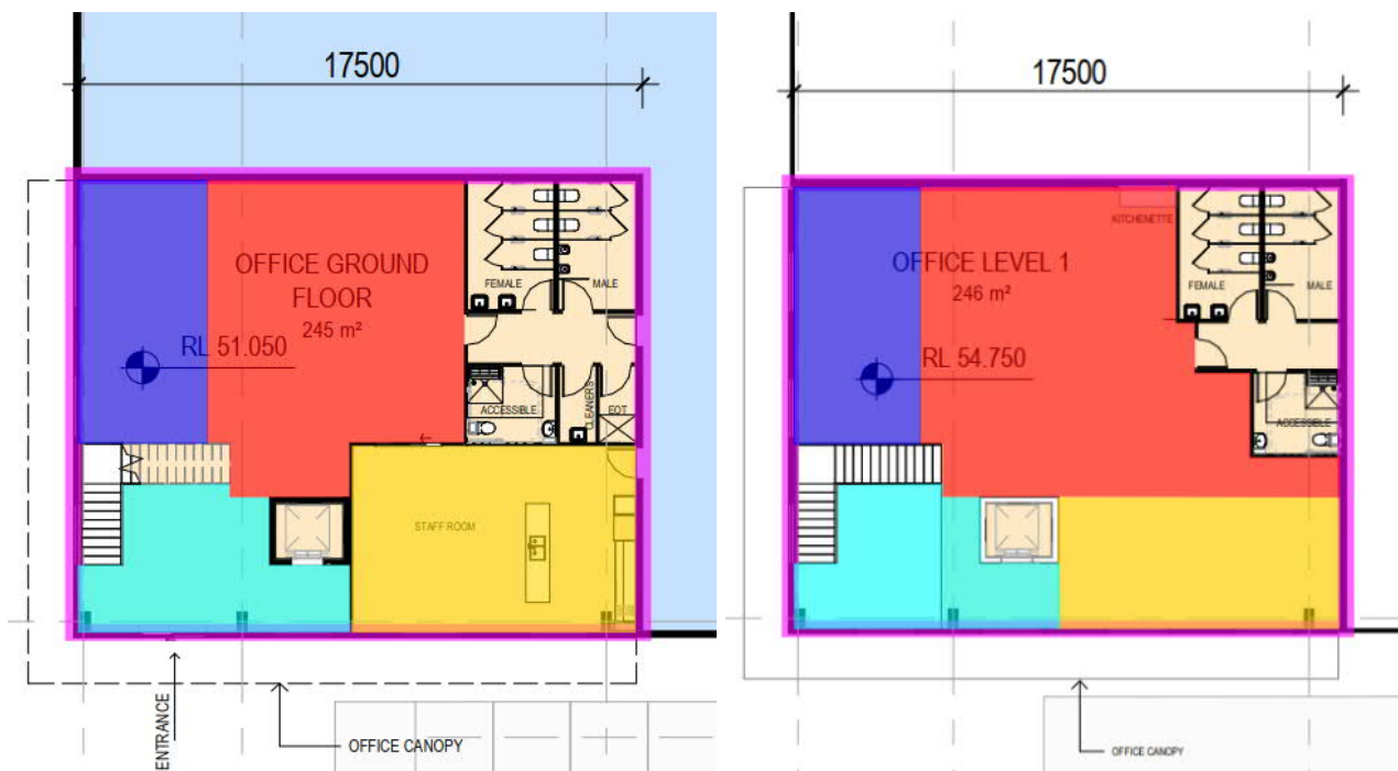
Figure 25: HVAC zones & thermal envelope for 8 McLaren Drive Ground Floor (Left) and First Floor (Right)
