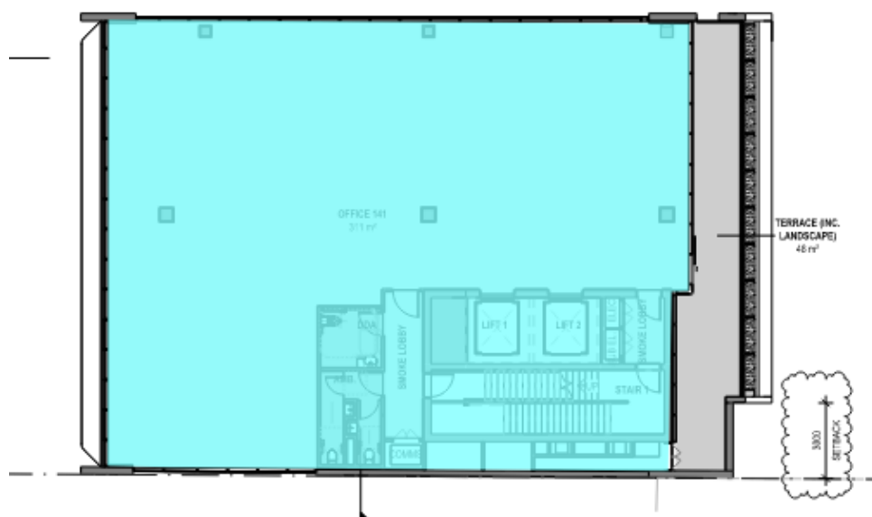
Figure 12 Conditioned space for level 14
