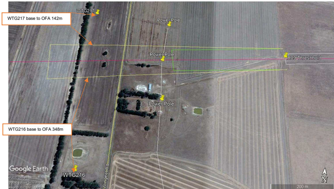
Figure 5 – Turbine distance to suggested obstacle free area
