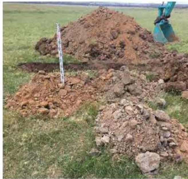
FIGURE C-6 TP110A – CLAY WITH BOULDERS TO 2.5 METRES (GOLDER, DEC 2019)
