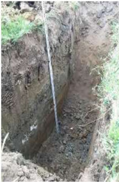
FIGURE C-6 TP110A – CLAY WITH BOULDERS TO 2.5 METRES (GOLDER, DEC 2019)
