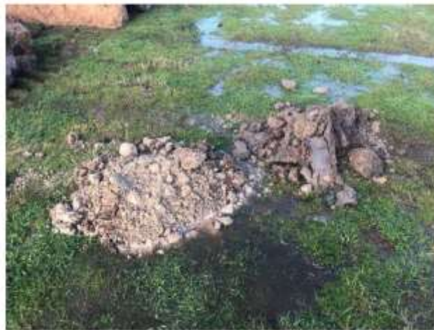
FIGURE C-8 PEDOLITH AREA AT TP165 NEAR MIA MIA CREEK SHOWING STANDING WATER THAT DOES NOT RAPIDLY INFILTRATE TO THE WATER TABLE
