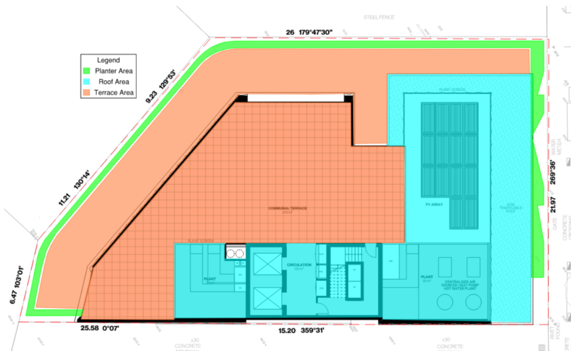
Figure 5 Site total stormwater catchment area
